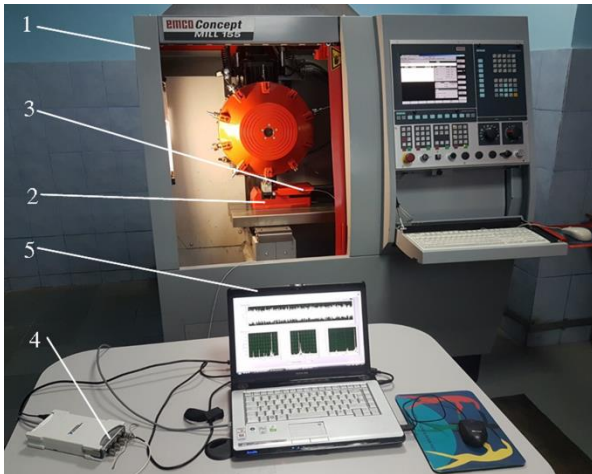
Figure 1. CNC machine and the vibration measurement system.
