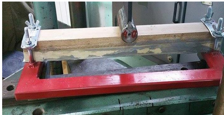
Fig. 2. Reinforcement application: two sheets of glass fiber fabric
