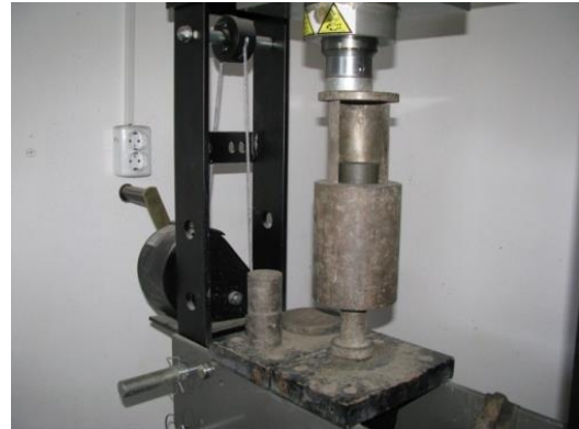
Fig.4. Manufacturing of ash samples
