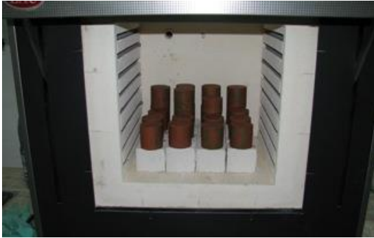
Fig.6. Burning the ash samples
