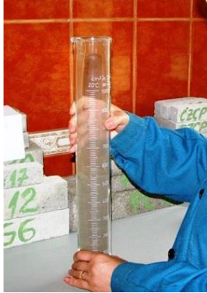
Fig. 2. Bulk density determination
