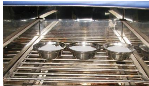
Fig.1. Drying process of the ash samples
