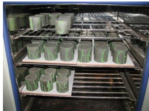
Fig.5. Drying the ash samples
