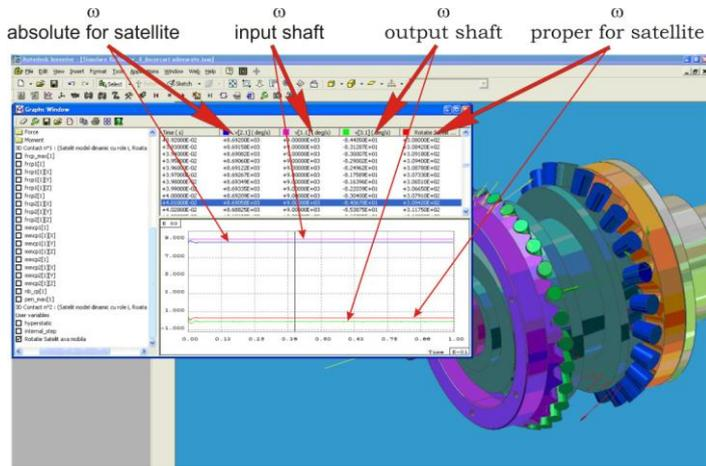
**Fig. 6.** Kinematic calculation of planetary precessional transmission.
