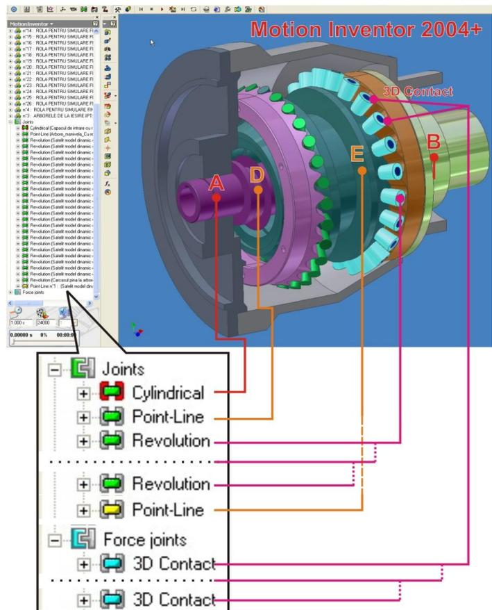
**Fig. 5.** Kinematics joints in the planetary precessional transmission.
