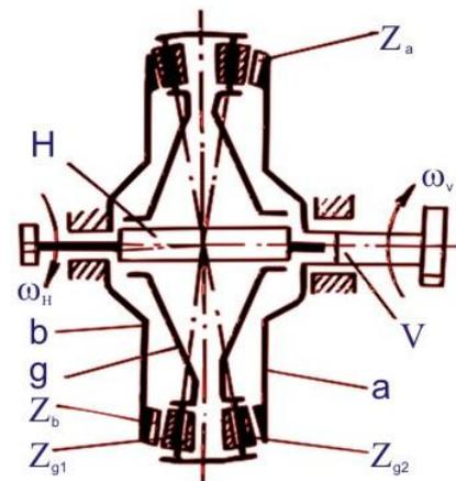
**Fig.1.** Kinematical scheme of planetary precessional transmission
