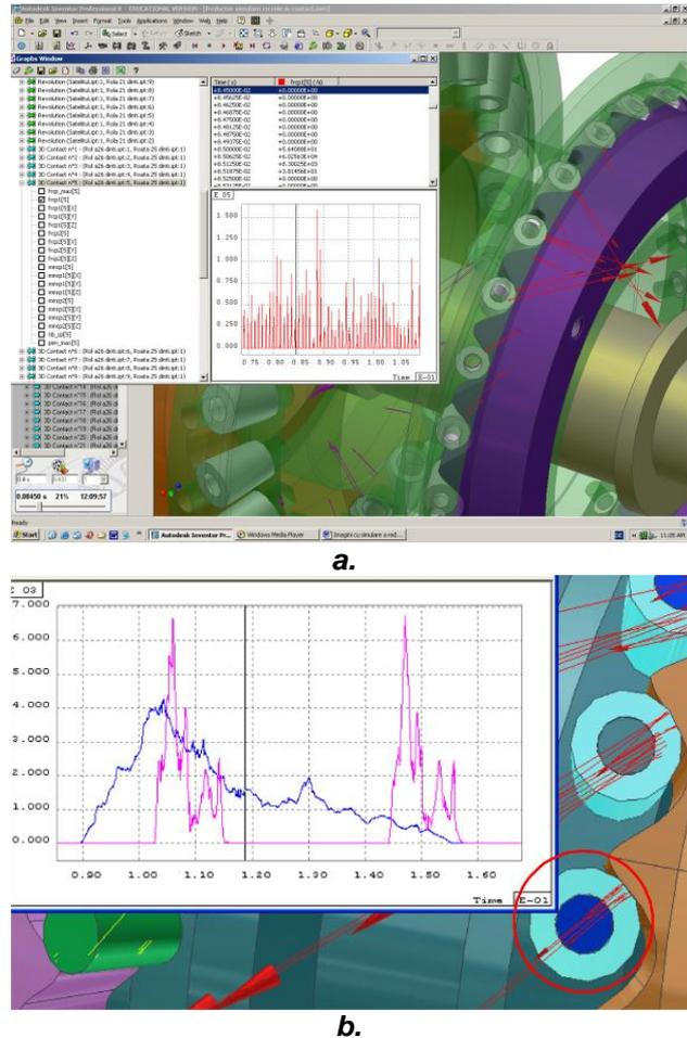
**Fig. 7.** Normal forces among the teeth and their distribution among simultaneously geared teeth
