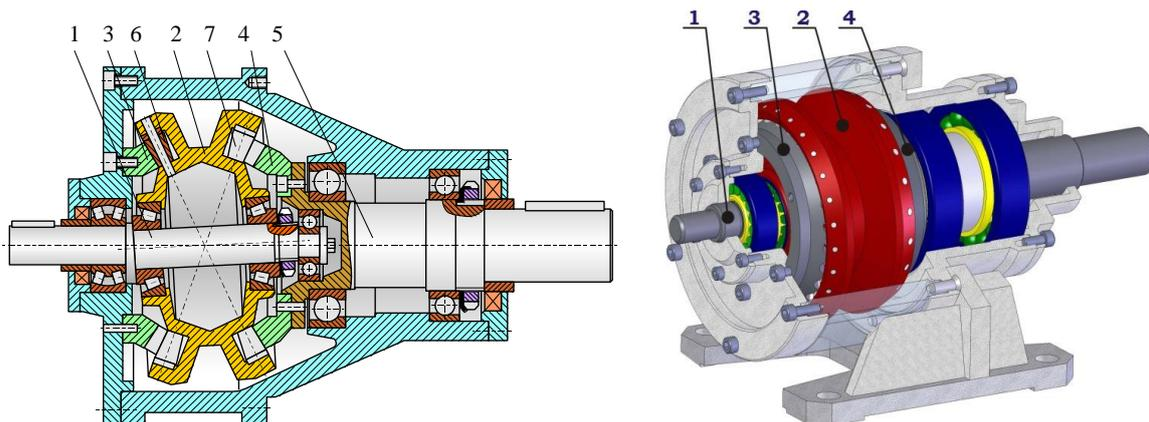
**Fig. 2.** Design of planetary precessional transmission
