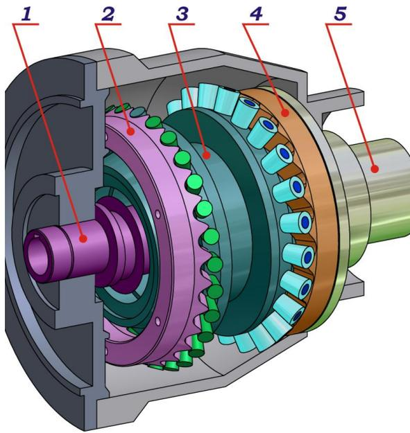
**Fig. 4.** 3D Model of planetary precessional transmission
