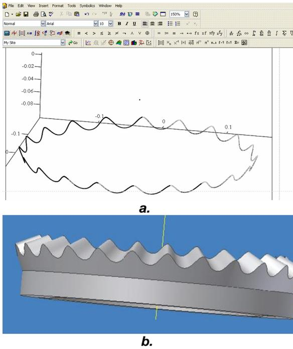
**Fig. 3.** 3D linear contour of central wheel teeth profile (a), and 3D model of the central wheel (b)
