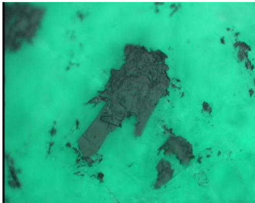
*Figure 2. Graphene flakes*
