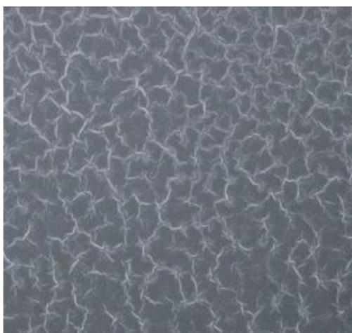
*Figure 3: Edge-functionalized graphene deposited on a silica substrate*
