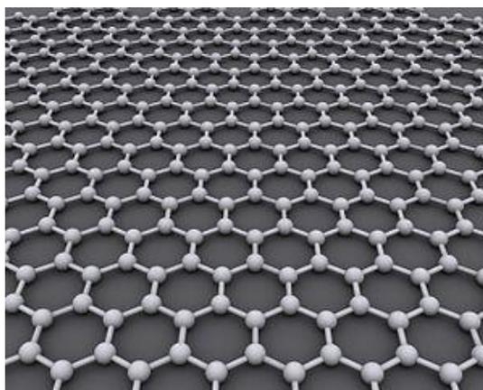
*Figure 1. Graphene – 1 layer graphite*
