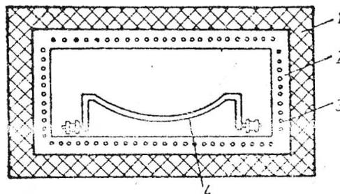
**Fig. 3.** Section through the furnace for curving through modelling:
