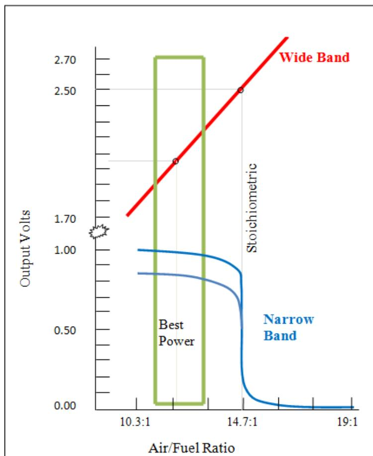
Figure1. Oxygen sensor output – narrow and wide band [11]
