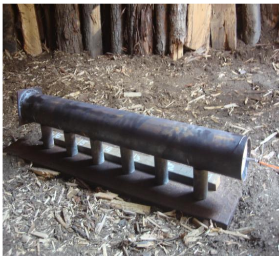
Figure 4. Blasting scheme for the detonability test for chemical fertilizer in bunker
