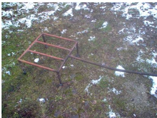
**Fig. 2** – Burner for test method for determination of flammability of the conveyor belts
