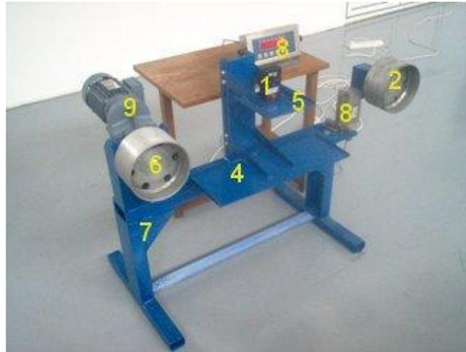
**Fig. 1** - Test stand for determination of the electrostatic field generated by a light transporting belt in operation
