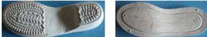
**Figure 3.** Burnt plaster cast
