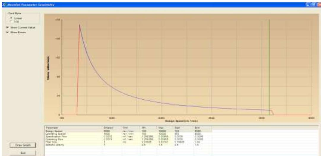
Fig. 5 Failures / million hours function according design speed
