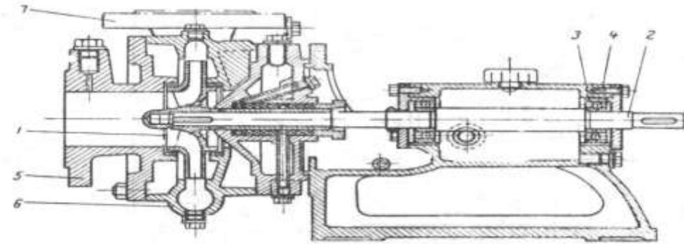
Fig. 2 Construction of centrifugal pumps
