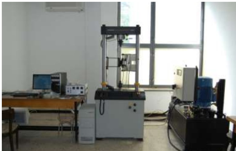
Fig. 4 The fatigue testing system INSTRON 8801.
