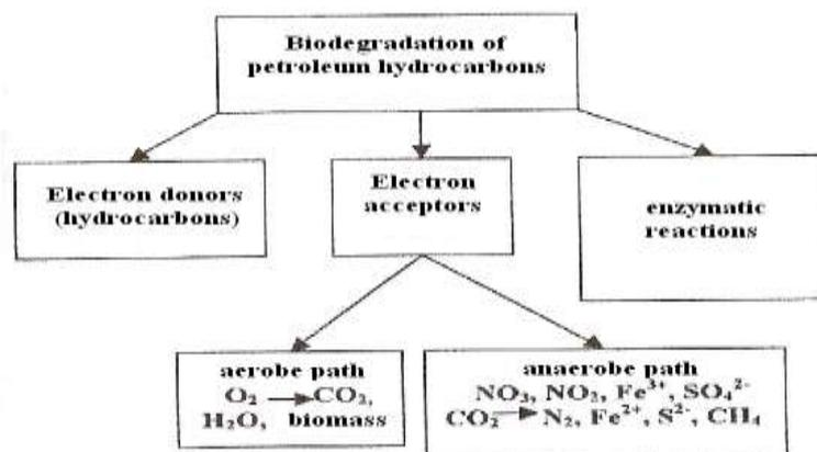
Fig. 1. Schematic representation of degradation processes petroleum hydrocarbons
