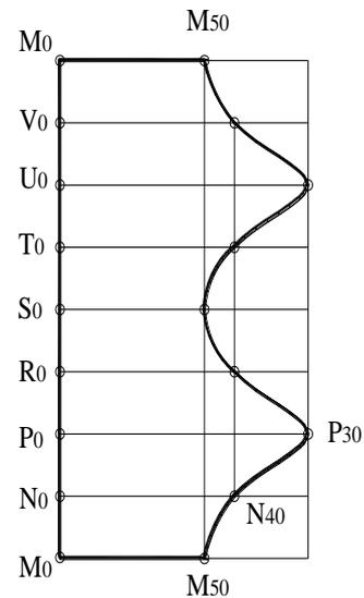
**Fig. 2.** Unfolding of the middle cylinder
