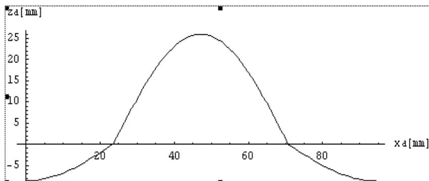
*Fig. 5. Unfolding of the horizontal cylinder*
