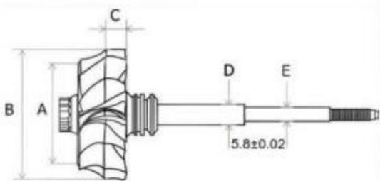
Fig.1. Turbocharger shaft.
