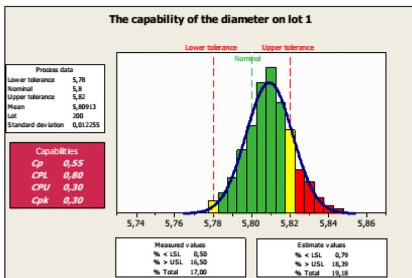
Fig.3. The capability of the diameter on lot 1.
