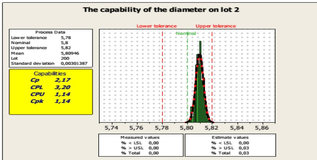
Fig.4. The capability of the diameter on lot 2.
