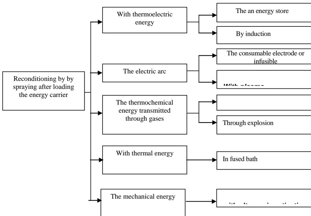
**Fig.1.** Classification by loading major for reconditioning processes by thermal spraying
