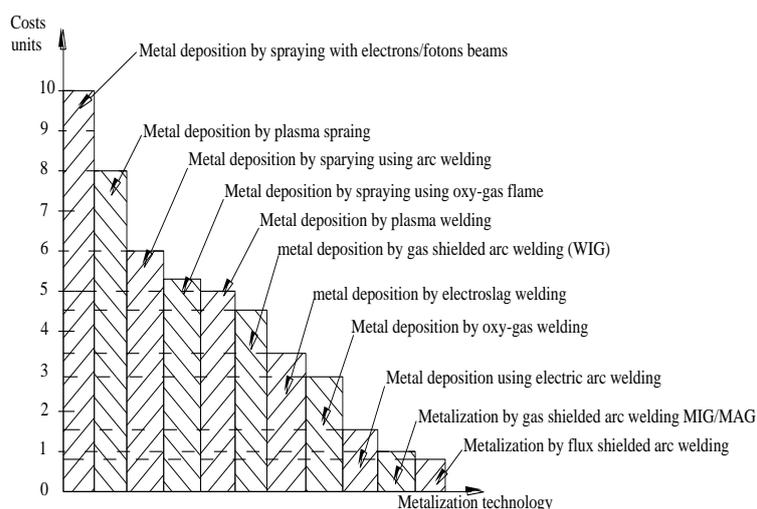
**Fig.2.** Relative costs based on unit mass of hard alloy charge deposited by different procedures
