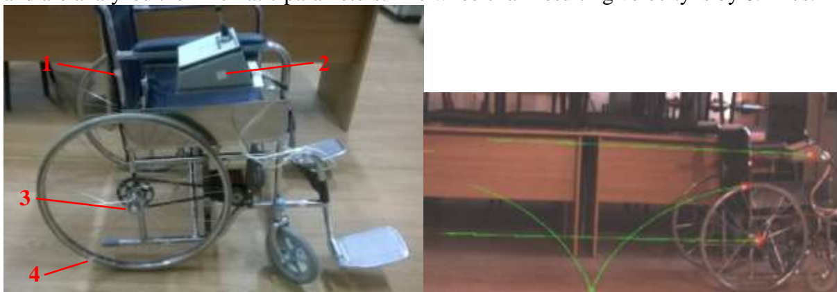
Fig.7. Positioning of reflective markers on the wheelchair and markers obtained trajectories.
