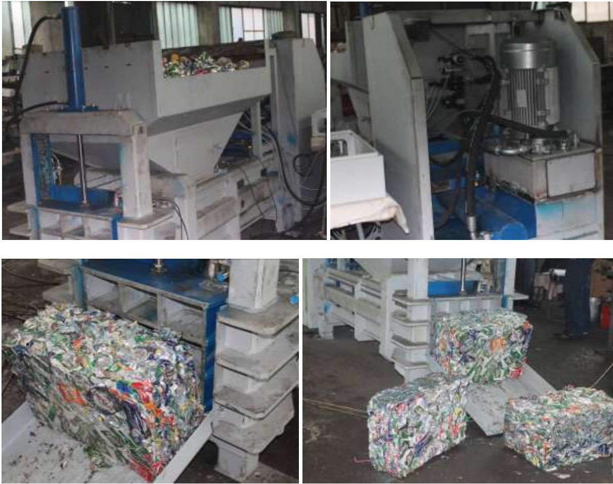
Fig. 12. Development and trials with Al box bundling press
