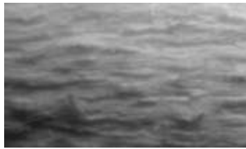
Fig. 7a The surface at f = 1.5 mm/rot Fig. 7b Detail
