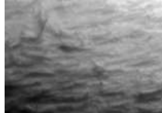
Fig. 8a The surface at f = 1.83 mm/rot Fig. 8b Detail
