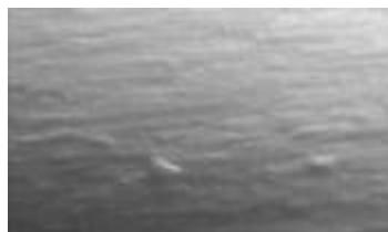
Fig. 3b Detail - the surface at f = 0.25 mm/rot
