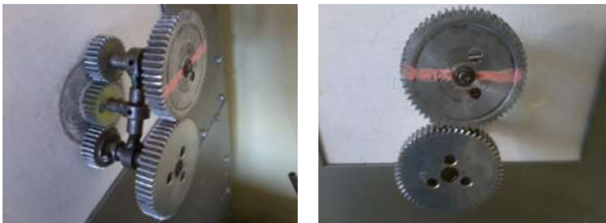
Fig. 8. Images foto of mechanism model with external cylindrical gearings
