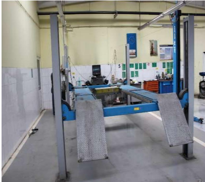
**Fig. 3.** Photo image of a car elevator with 4 poles – upper position [10]
