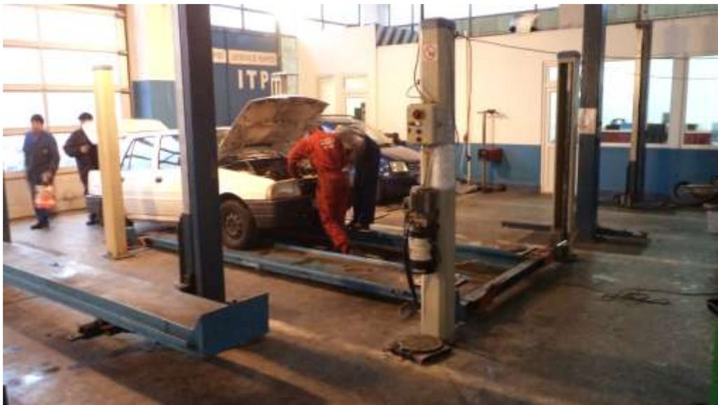
**Fig. 4.** Photo image of a car elevator with 4 poles (simultaneously actuated by means of a cable), in the lower position (on the ground)
