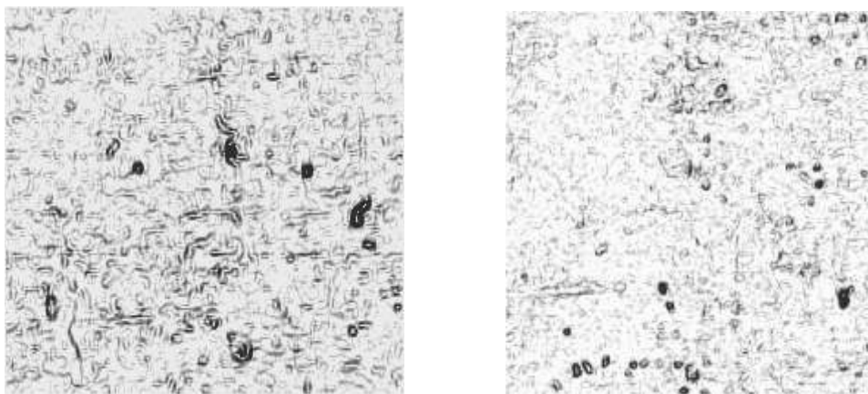
Fig.3.b Traces of wear F = 250N , N_c = 40,000 cycles - lower blade
