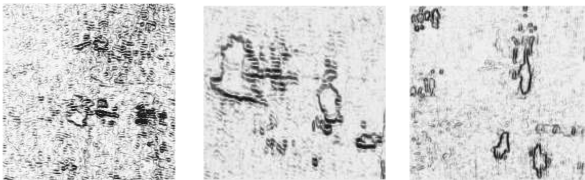
Fig.5.a Traces of wear F = 250\text{N} , N_c = 60,000 cycles - upper blade
