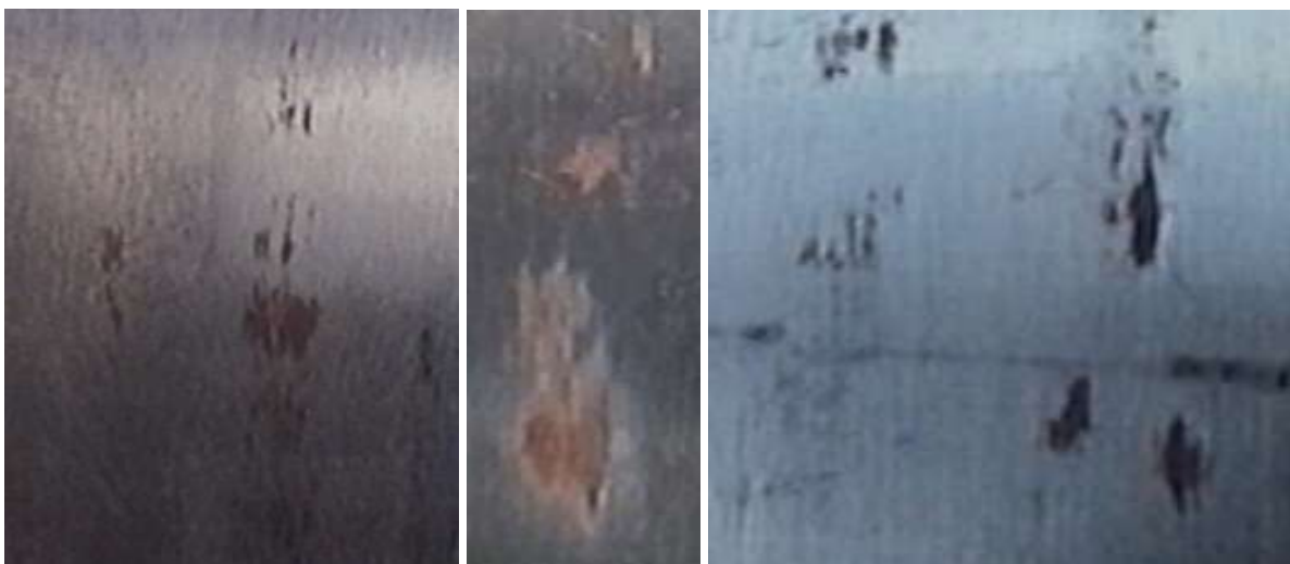
Fig.10 Traces of fretting for a normal load of 250N and 60000 load cycles
