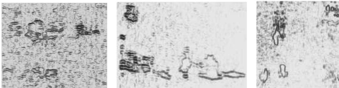
Fig.5.b Traces of wear F = 250\text{N} , N_c = 60,000 cycles - lower blade
