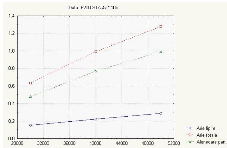
Fig.2. The dependence of the wear traces by the numbers of cycles for F= 200N; in front
