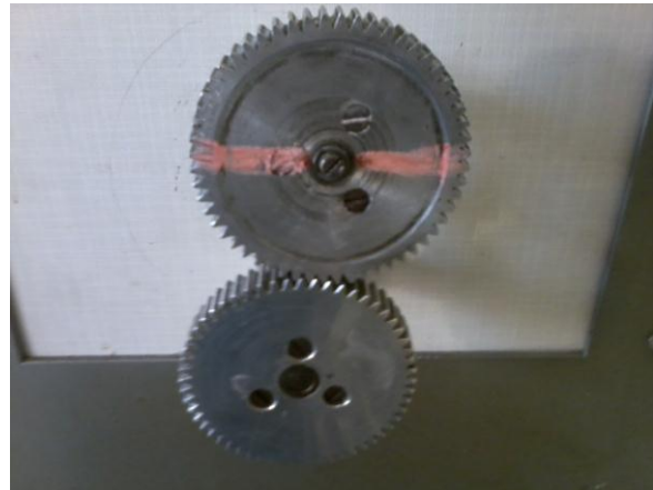
Fig. 8. Images foto of mechanism model with external cylindrical gears
