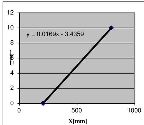
Fig.8 Transducer transfer characteristic
