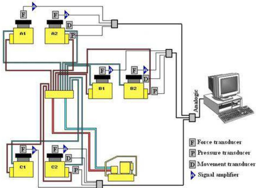
Fig. 4 Transmitter data collection system – analogical signal
