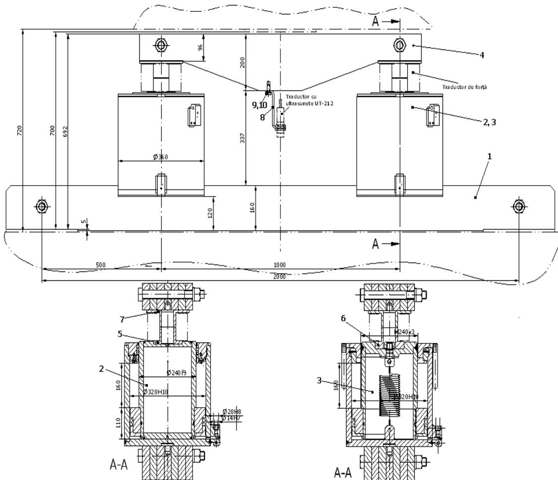
Fig.2 General view of the lifting installation
