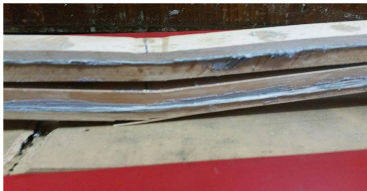
Fig. 3 Testing a reinforced ash wood beam with two GFRP sheets and two slides of beech wood (up and down)
