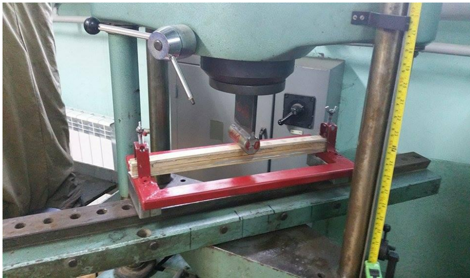
Fig. 1 Testing a reinforced wood beam with one GFRP sheets
