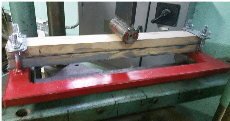
Fig. 5 Testing a reinforced ash and beech wood beam with one GFRP sheet (in the middle of the beam)
