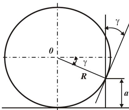
Fig. 1. The design scheme of the parameters of the microcutting process with a unit grain
