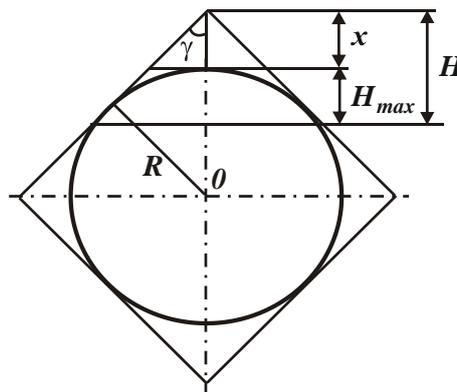
Fig. 2. The design scheme of the parameters of the microcutting in grinding process
