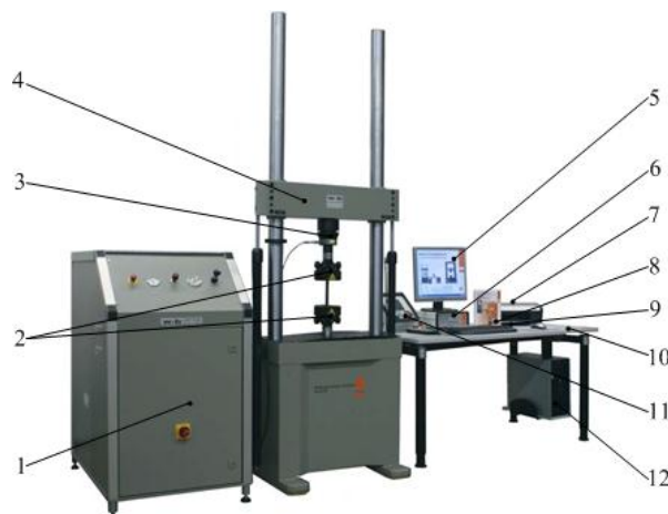
Fig. 3 The Components of the fatigue test machine
