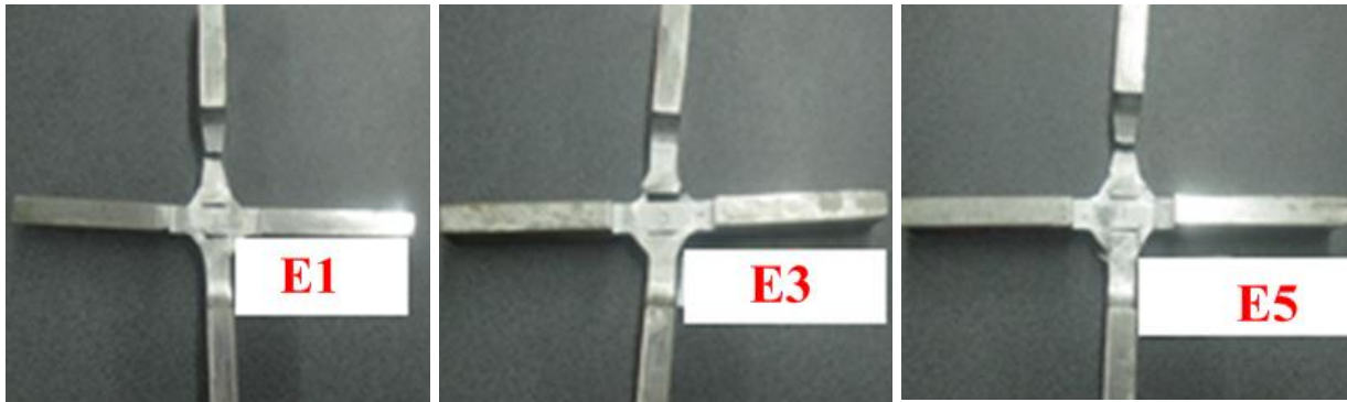
Fig. 4 Fatigue test specimens variable loaded
