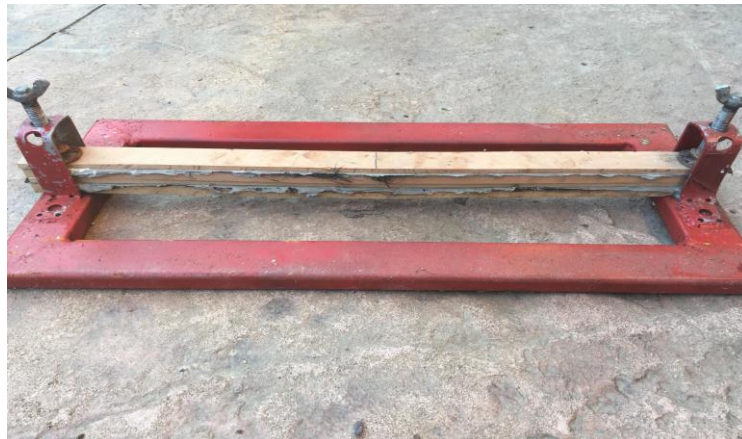
Fig.2 Reinforced wood beam (Type B)
