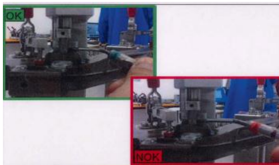
Fig. 7. Visual aid for checking position deviation in Y of the M10 x 1.25 nut
