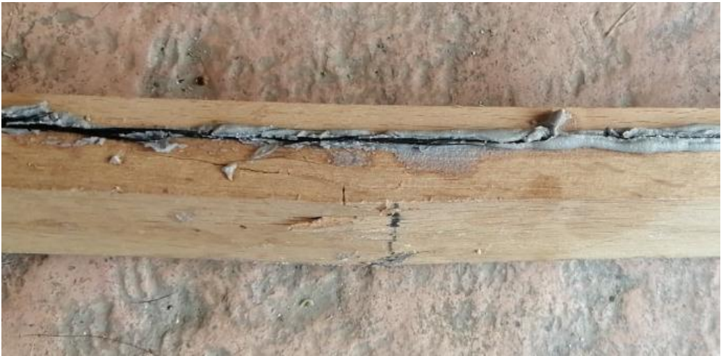
Fig 3. The beams after bending test
