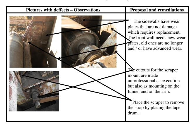
The upper spill bulkhead on the conveyor, to the conveyor underneath the car that transports it to crush and further into the bunkers that feed the boilers of the thermoelectric plant, has the role of directing the coal in the desired direction. It is located at the end of the conveyor belt in the immediate vicinity of the drive drum trapped on the rotating platform.
