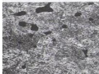
Fig.1. Microstructure of Astaloy A+ 0,25% C
