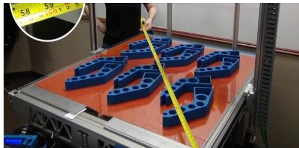
Figure 3. Multiple objects can be placed without additional space in the 3MF file format
