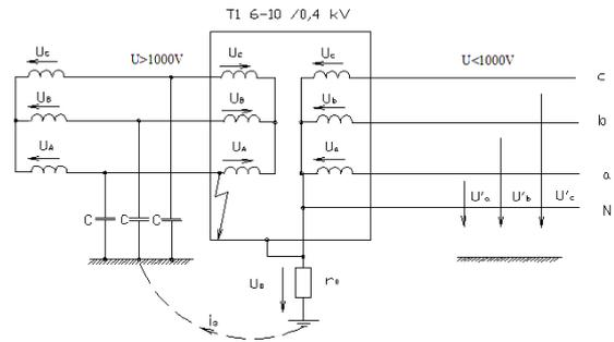
Figure 1. Equivalent circuit diagram of electrical power network for studying the emergency mode of a power transformer 6(10)/0,4 kV in case of insulation break-down between the high-voltage winding and the transformer frame, where:
