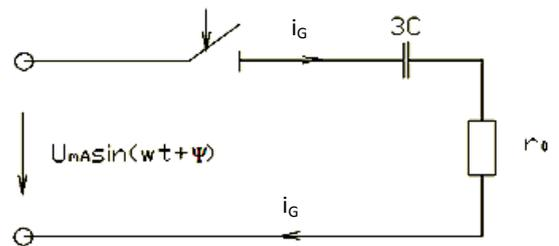
Figure 3. Calculation circuit of the electrical power line.
