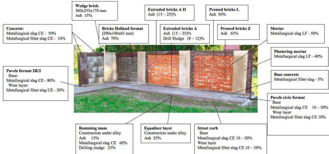
**Figure no. 3. Experimental wall that containing some kind of bricks, pavers, bordures, mortar and concrete, obtained within LIFE ENV 729 RO Project**
