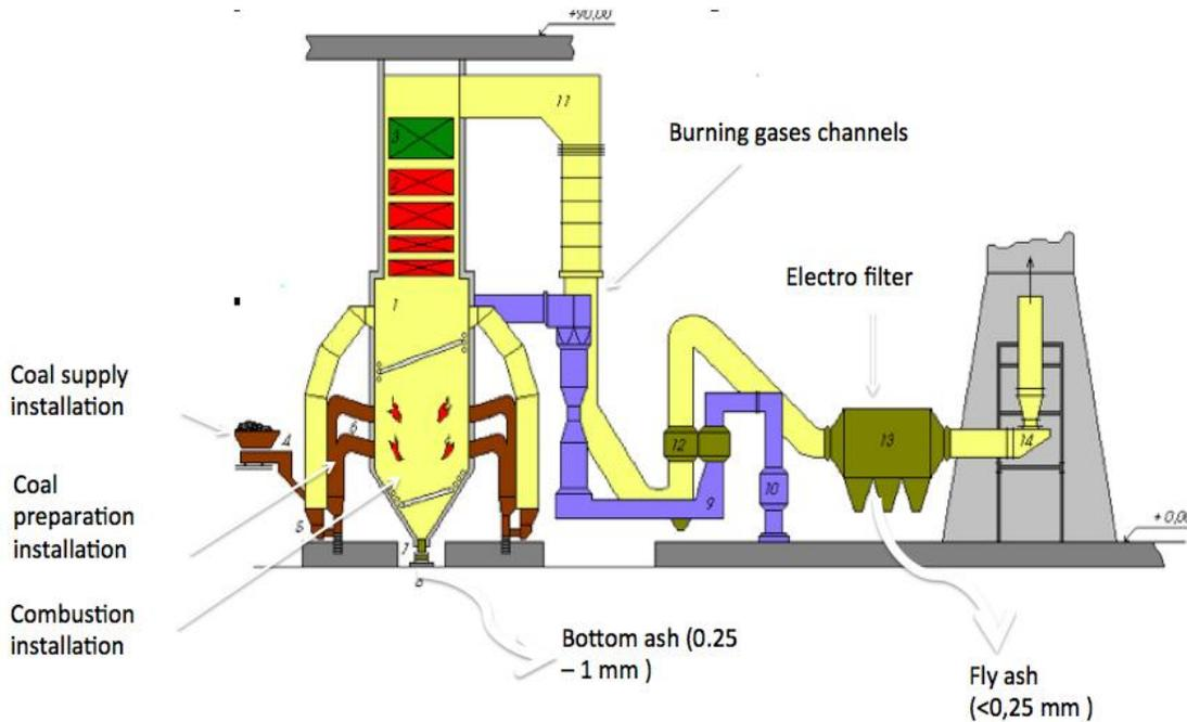
Figure no. 1 Ash generation in thermal power plant
