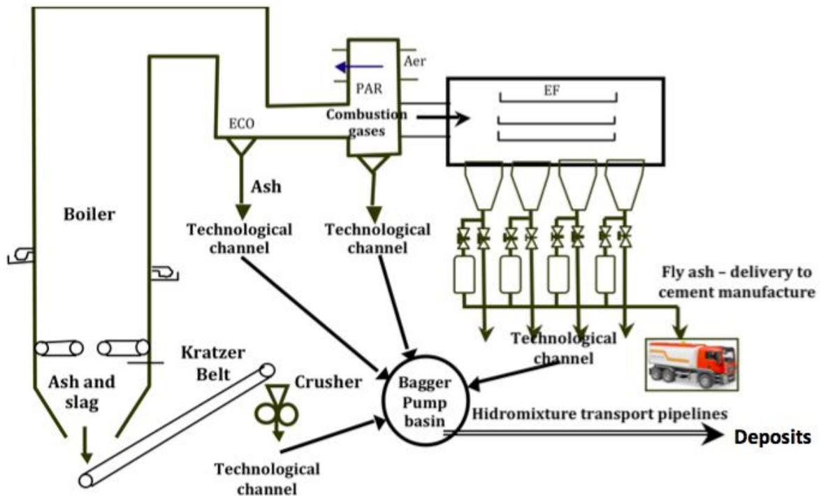
Figure no. 2 Ash and slag disposal in thermal power plant
