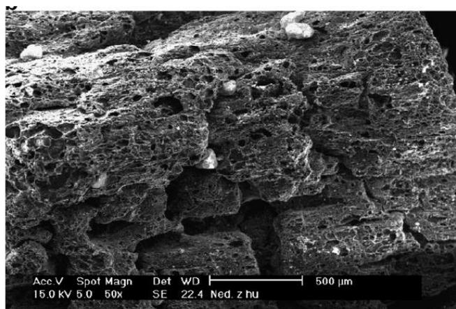
Figure 1. SEM photograph of unburned carbon from bottom ash obtained from lignite [5]
