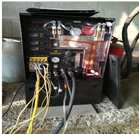
Figure 3. The emission sampling equipment
