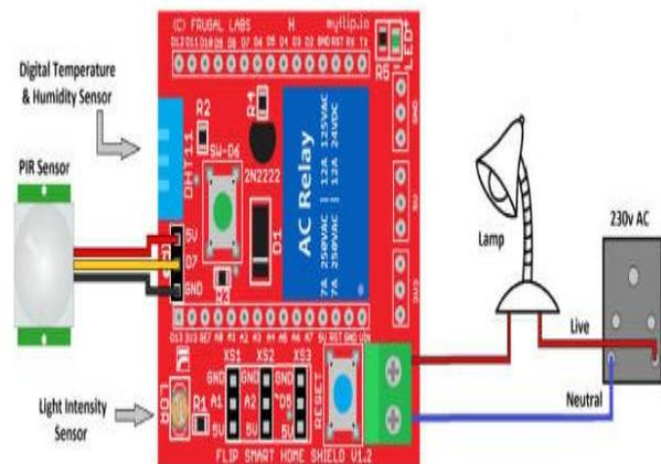
Figure 3. Smart Home Device Setup
