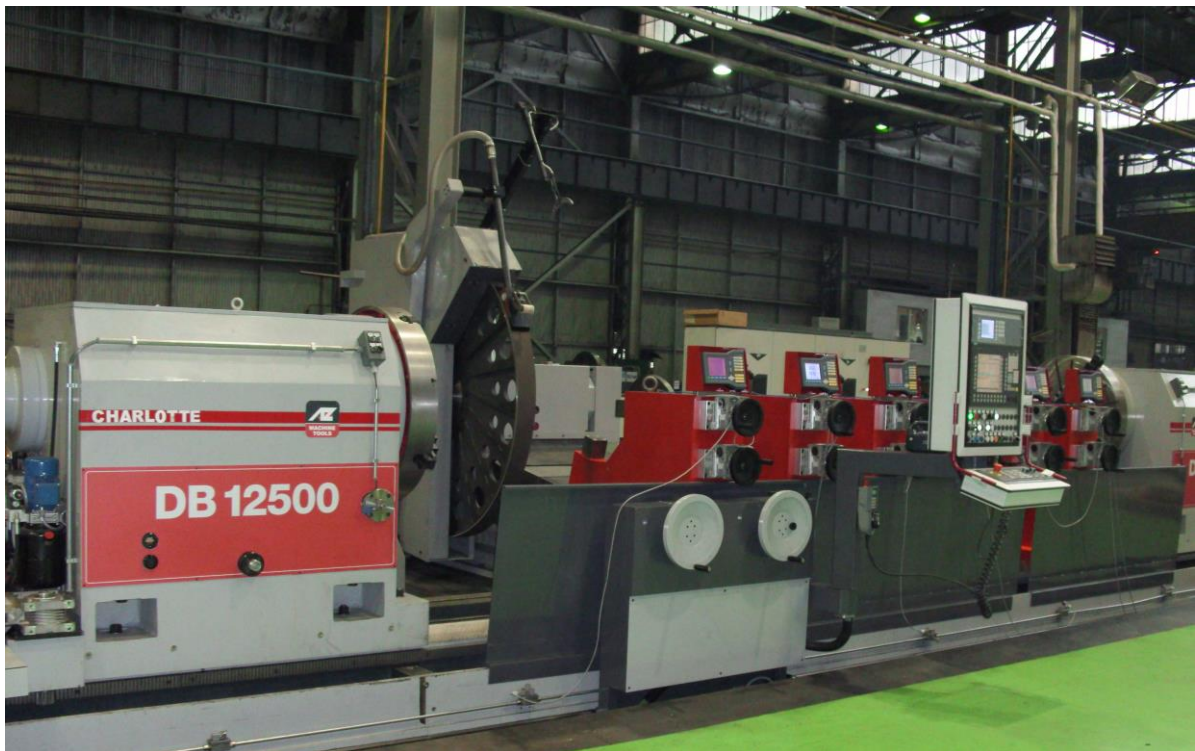
Fig. 1. The DB12500 grinding machine
