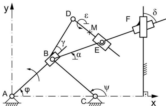
Fig. 1. The mechanism analyzed
