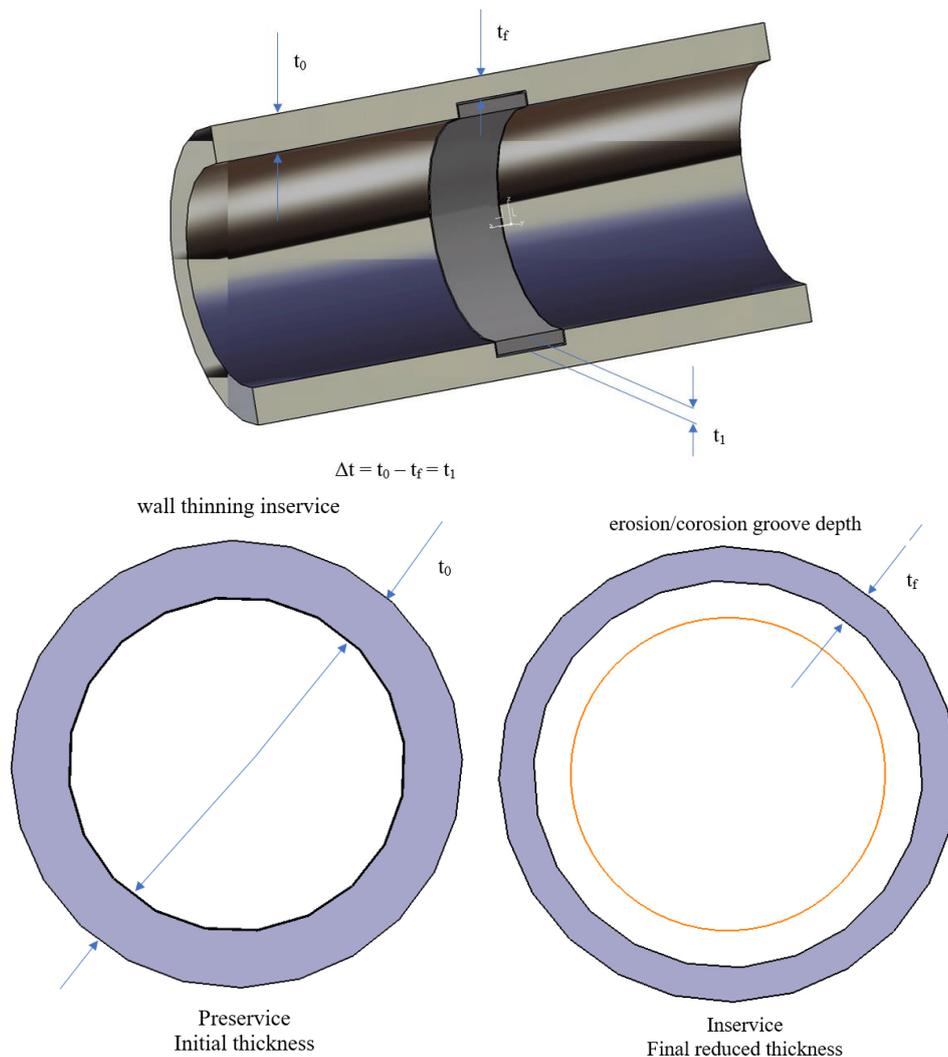
Fig.1. Defects that occur during erosion / corrosion
