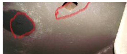
Picture 4. Cuts in the lower plate.
