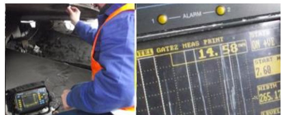
Picture 7. Thickness control of tripod plates
