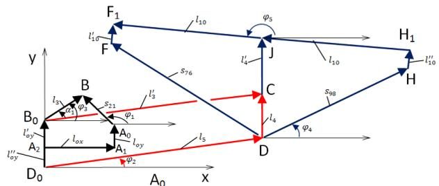
movements. Even though we have three cylinders, two of them (6,7 and 8,9) cannot work at the same time – when one is active, the other one is passive or in another words one cylinder drives the other one.
