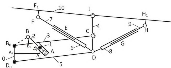
**Figure 4.** Structural / Vectorial schematic of the lifting / tilting mechanism
