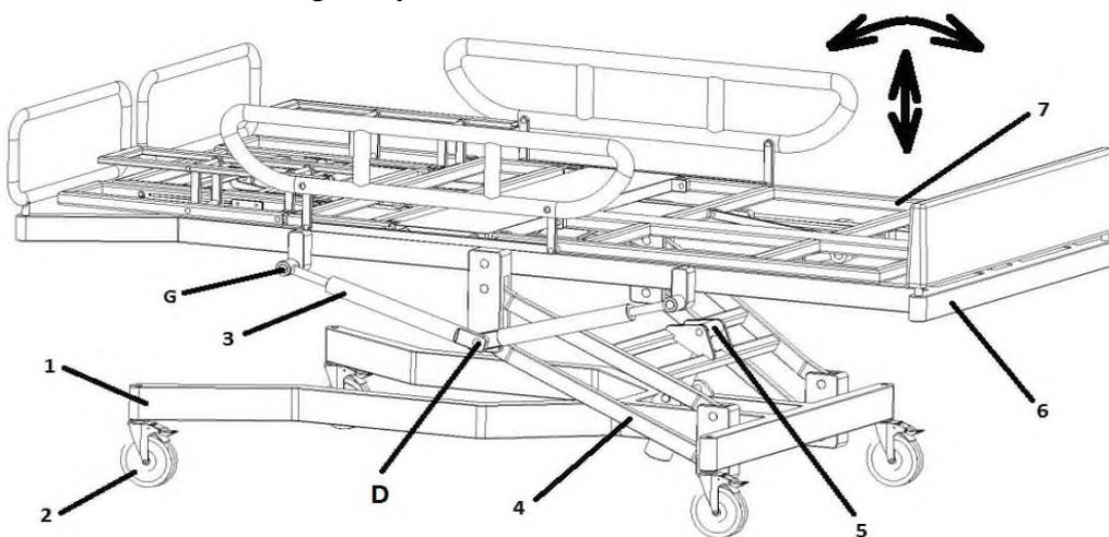
**Fig. 3.** Lifting and tilting patient support platform mechanism – 3D model
