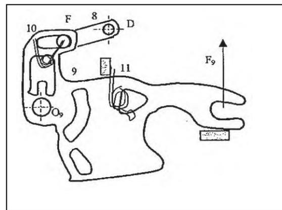
**Fig. 9.** Inside latch release and lock/unlock levers
