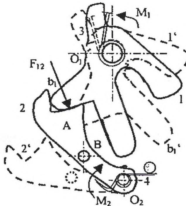
Fig. 7. Kinematical schema of a catch/pawl interface –closed and open (dotted line)
