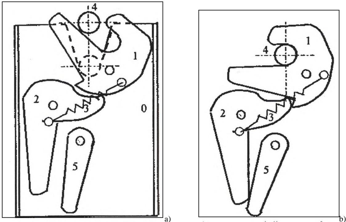
Fig. 4. Typical components of a decklid latch – open (a) and closed (latched) position (b)
