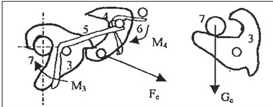
Fig. 1. Kinematical representation of a hood latch mechanism
