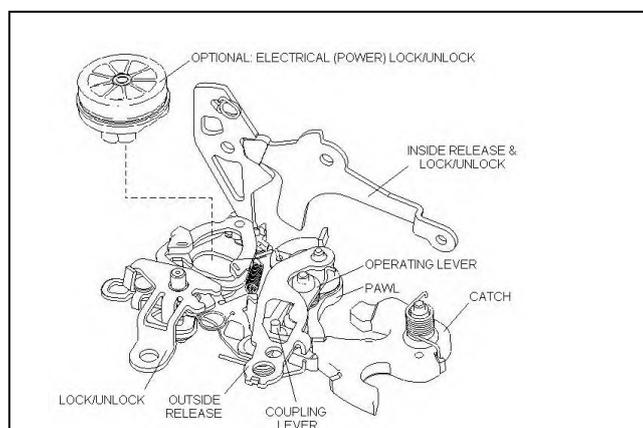
Fig. 5. Isometric view of the catch release chain (Ford-NGL2)
