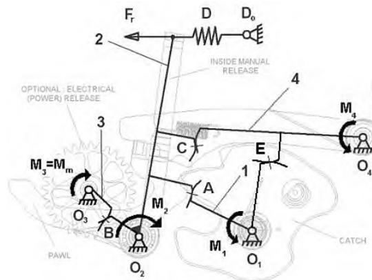
Fig. 11. Constructive and kinematical scheme of lift mechanism
