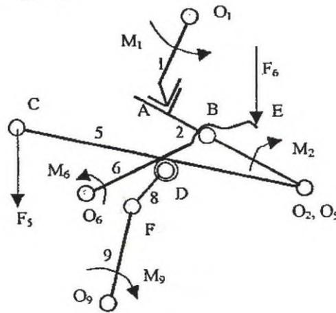
Fig. 10. Kinematical scheme of a side door latch
