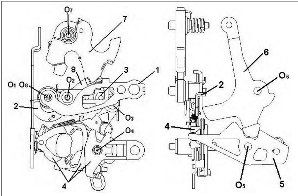
Fig. 6. Catch release chain – side door latch (Ford-NGL2)
