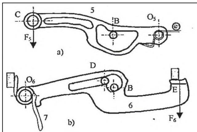
**Fig. 8.** Outside latch release: lever inside the latch (a) and outside (b)
