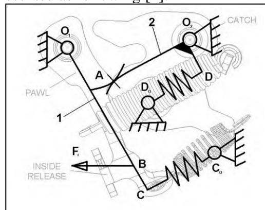
Fig. 3. Hood latch kinematical scheme
