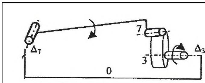
Fig. 2. The spatial hood latch mechanism.
