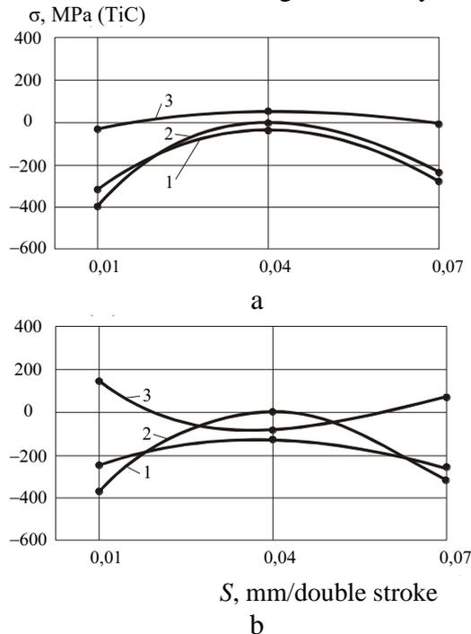
Fig. 3. Influence of traverse on residual stresses in TiC and Ni phases.
