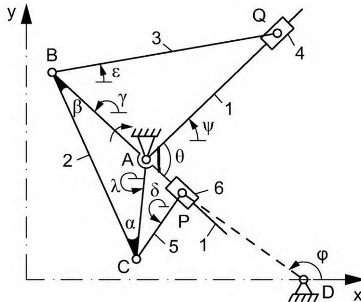
Fig. 3. The Sylvester-Kempe reversing mechanism
