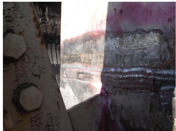
Figure 3 - Lack of microcracks in visual verification
