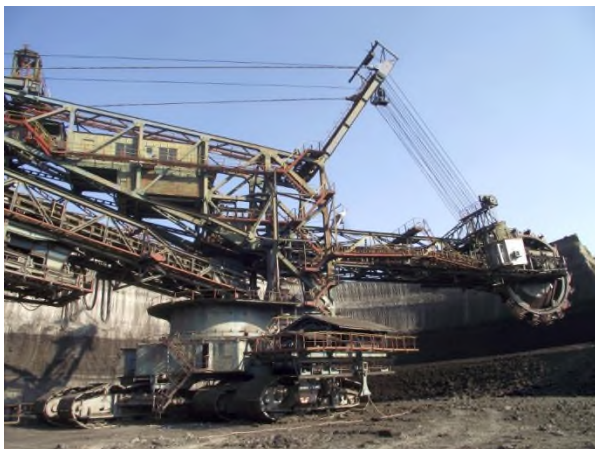
Figure 1 - The excavator with rotor type ERc 1400-30/7
