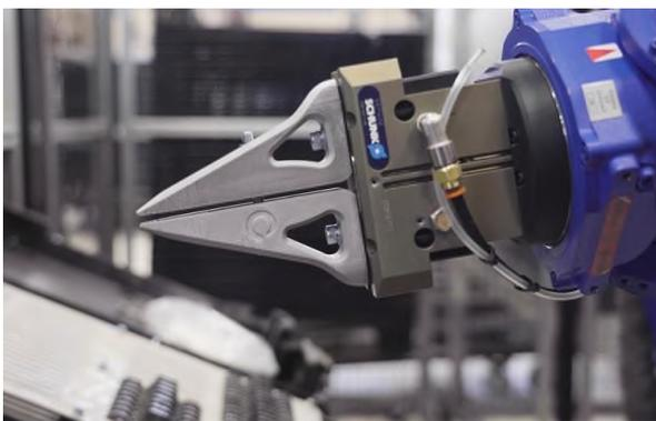
**Figure 2.** 17-4 PH Stainless Steel grippers, 3D printed [13]
