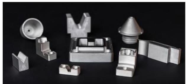
**Figure 4.** 3D printed parts made of H13 Tool Steel [13]
