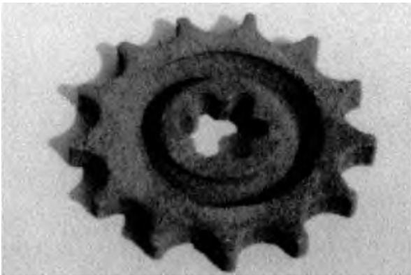
**Figure 1.** First metal part created using 3D printing [9]
