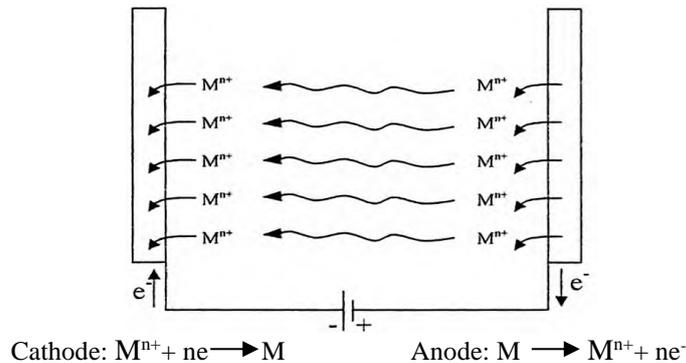
Fig.1. Schematic diagram of electrolytic deposition
